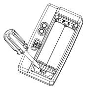
2. Use a flat-blade screwdriver to push the button located in the hole for around three seconds.
