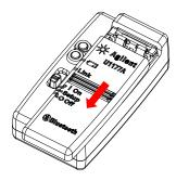
1. Slide the battery cover away from adapter's body.
