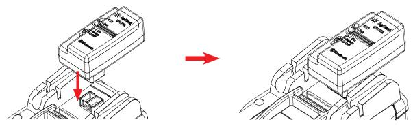
Snap the optic side of the U1177A to the multimeter IR communication port.
