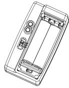
1. Open the battery cover. Then, set the slide switch to **Setup**.
